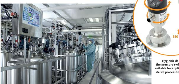
Hygienic design: the pressure switches are suitable for applications in sterile process technology
