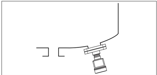
Fig. 14: Measurement setup for the level measurement
