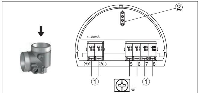
Fig. 18: Electronics compartment - double chamber housing
