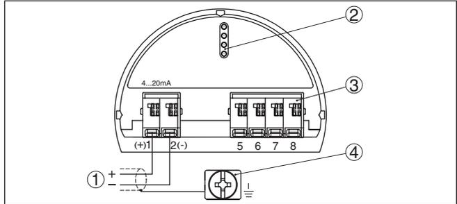
Fig. 17: Electronics and connection compartment - single chamber housing
