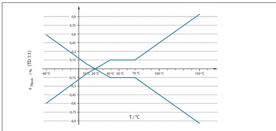
Fig. 33: Basic temperature error  $F_{TBasis}$  at TD 1 : 1
