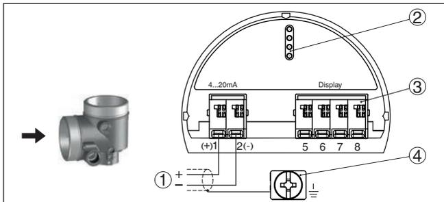
Fig. 19: Connection compartment - double chamber housing
