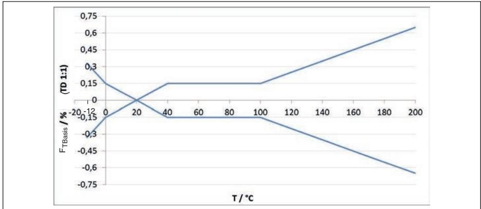
Fig. 34: Basic temperature error  $F_{TBasis}$  at TD 1 : 1
