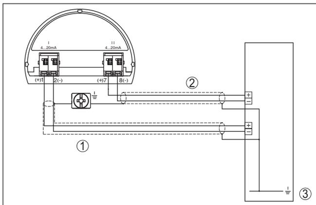
Fig. 37: Connection example DPT-20 additional current output
