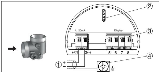
Fig. 29: Connection compartment - double chamber housing
