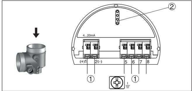
Fig. 31: Electronics compartment - Ex-d double chamber housing
