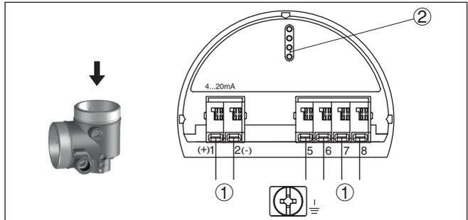
Fig. 28: Electronics compartment - double chamber housing
