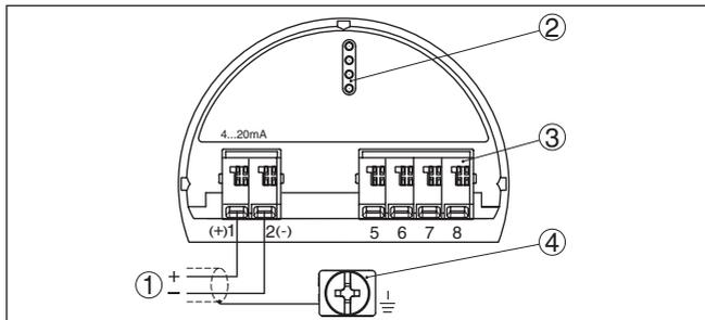
Fig. 36: Electronics and connection compartment - single chamber housing
