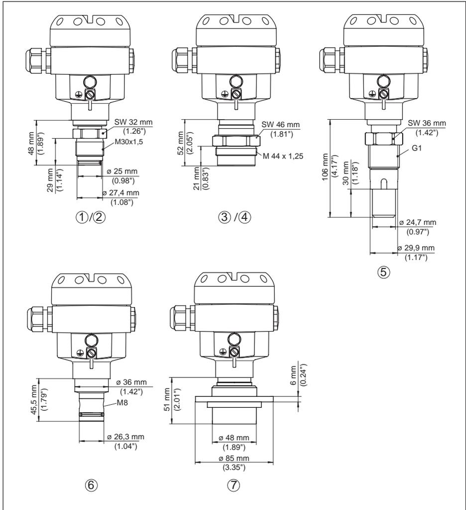
Fig. 43: CPT-2x, racor tubular
