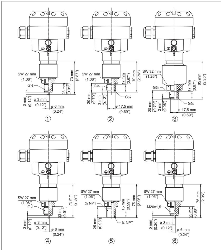
Fig. 39: CPT-2x, racor roscado no rasante
