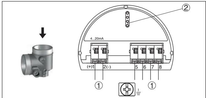
Fig. 23: Electronics compartment - double chamber housing
