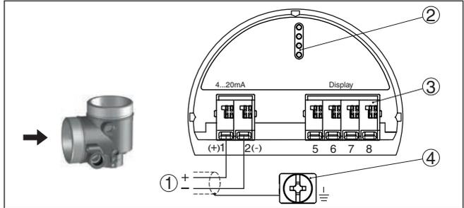
Fig. 24: Connection compartment - double chamber housing
