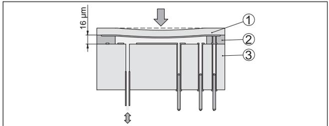
Fig. 3: Configuration of the ceramic measuring cell
