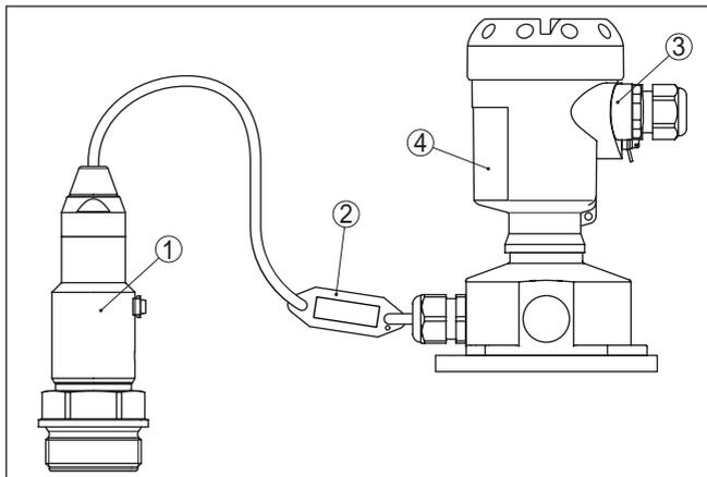
Fig. 20: Combination process assembly and external electronics
