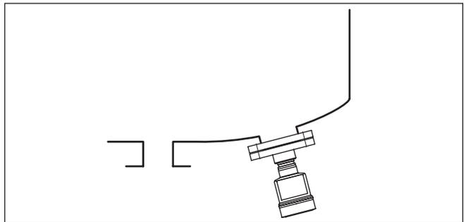
Fig. 18: Measurement setup for the level measurement
