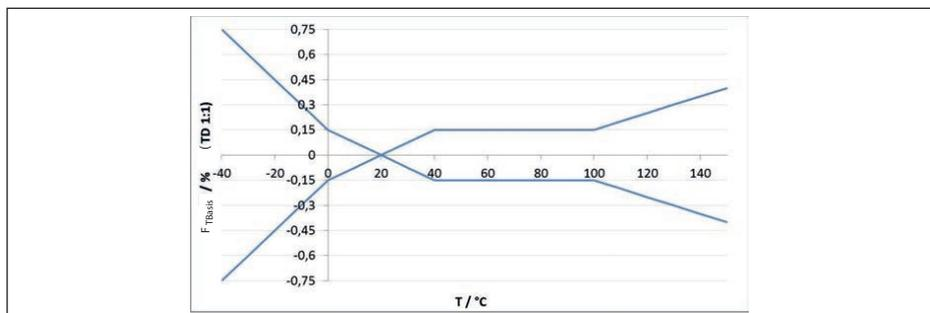
Fig. 39: Basic temperature error  $F_{TBasis}$  at TD 1 : 1
