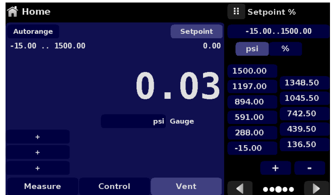
Figure 6.4.1.2.3-B – DUT Pressure Value Entry
