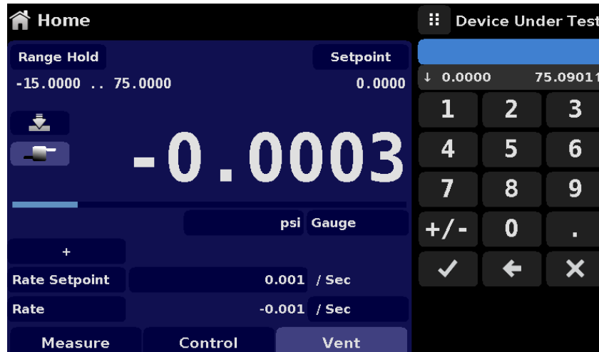
Figure 8.6.3-C - DUT pressure for purge sequence
