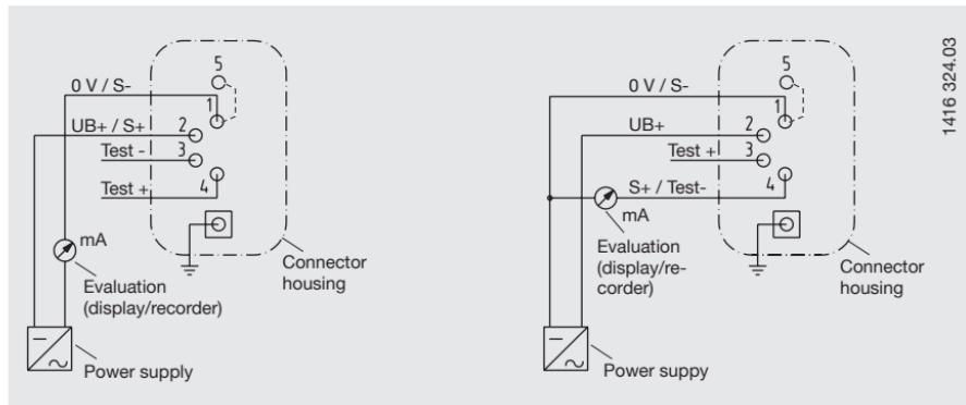
The transmitter can operate using a non-stabilised supply voltage within the given limits, so long as the voltage available to the transmitter does not fall below 10 V, or below 14 V for the LCD-display version.
