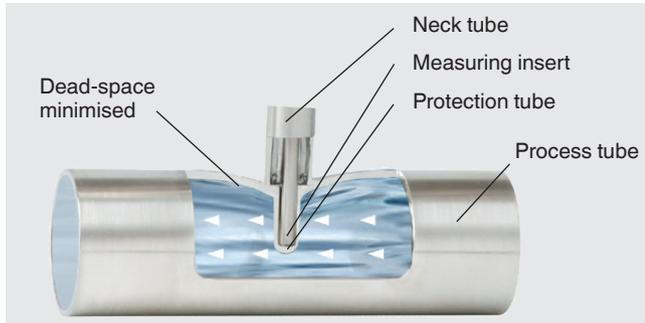
The patented hygienic design of the TW61 flow-through housing enables dead-space minimised, invasive temperature measurement and, through self-draining, a flexible mounting position.
