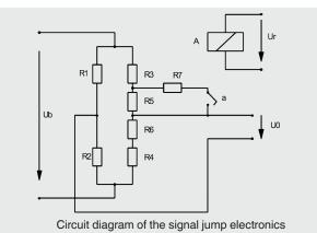
With these force transducers, four variable resistors (R1 ... R4) are connected together to form a Wheatstone bridge. When the measuring body deforms, the opposing resistors are stretched or compressed in the same way. This leads to a detuning of the bridge and a diagonal voltage U0.
