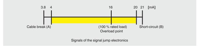
With a fixed signal jump of, for example, 4 mA, the test cycle can then be triggered, in any operating state, by activating the test relay. The upper measuring range limit of 20 mA will never be reached and thus the checking of the signal jump is enabled.
