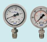
The 230.15 is the right choice for specialty gas, Ultra High Purity, PV and SEMI applications in gas distribution systems using face seal fittings. The 230.25 is best suited for applications that require VIM/VAR wetted parts and face seal fittings. Both product variants have electropolished media-wetted stainless steel surfaces, as well as electropolished stainless steel cases.
