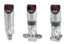
Optional alarm contacts are available for programming two user-defined switch points The WUD-2x incorporates a local, rotatable, and programmable display with the state-of-the-art electronics of the WU-2x. The WUD-2x transducer with integrated display provides a local reading of the process pressure measurement as well as the associated analogue output signal (current or voltage) from the transducer.
