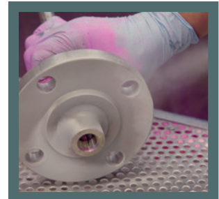
Liquid penetrant inspection
