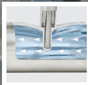
Representation of the flow conditions for a dead-space free thermowell vs. conventional design with collaring
